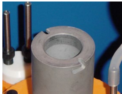
Figure 19. Engagement slots for bayonet fittings
