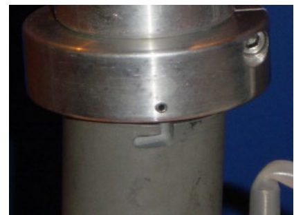
Figure 22. Correct orientation of motor on drive shaft
